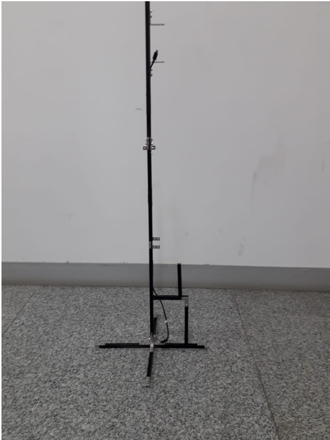
Figure FC3.2: Picture of an Aluminium stand made from Makerbeam extruded Aluminium beams. The Raspberry Pi is fixed at the top, while a Power Bank used to power is secured at the bottom. The Raspberry Pi is encased when using this stand to prevent Electrical Short-circuits as it's backed against metal.
